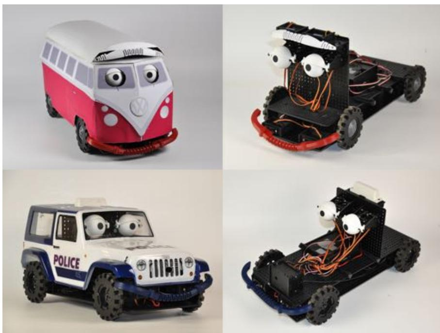
**Fig. 5.2** OTO – a mobile extension for the Opsoro platform
