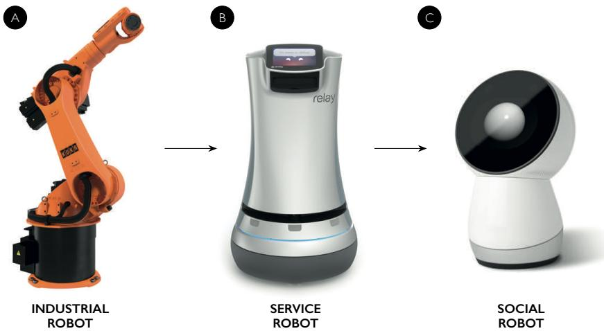
**Fig. I.16** Three types of robots: (A) industrial robots, e.g. KUKA robot arm, (B) service robots, e.g. Savioice Relay, (C) social robots, e.g. Jibo.
