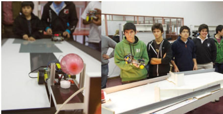
**Fig. 3.8** Playfields used during the contest. The left playfield has a light-to-dark gradient on the floor to guide robots toward the flame. The right playfield has a bright spotlight above the flame to aid the robots in navigation.
