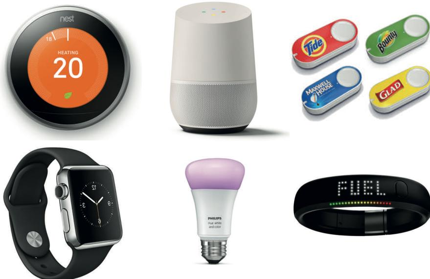
**Fig. 1.15** Examples of commercial Internet of Things (IoT) products. Starting from the top left and moving clockwise, they are: Nest thermostat, Google Home, Amazon Dash, Nike Fuel, Philips Hue, Apple watch.
