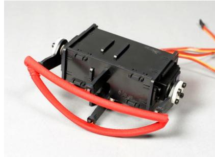
**Fig. 4.2** Mouth module prototype
