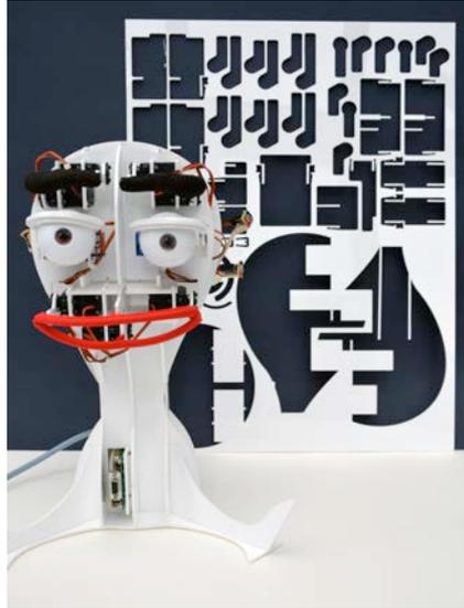
**Fig. 3.** Prototype with one of 2 laser-cut sheets in the background
