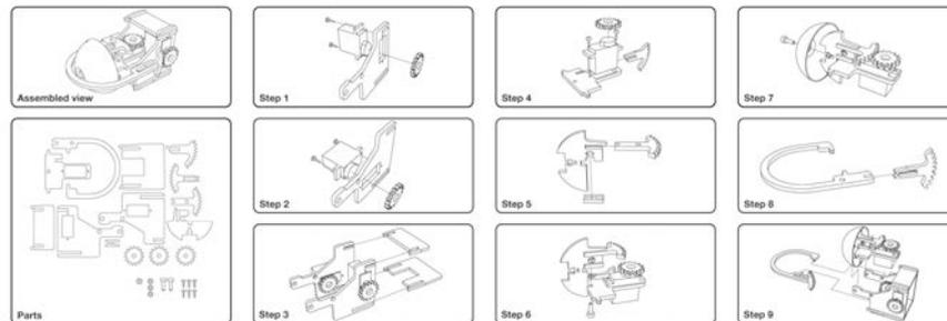
**Fig. 5.** Assembly instructions for an eye module
